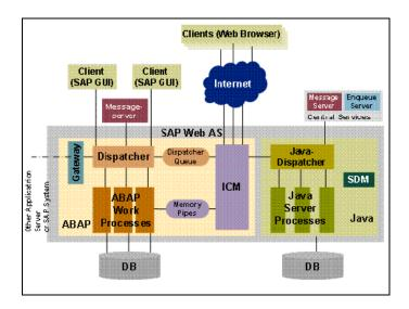
The above image illustrates the architecture of the SAP NetWeaver application server which includes both the ABAP and Java stack. Note that the two stacks can be installed separately or together.
